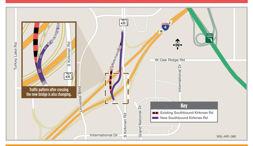
This long-term traffic pattern of approximately a quarter-mile in length will relocate the southbound lanes of Kirkman Road to a newly constructed bridge over westbound I-4. The new traffic pattern is necessary for the reconstruction of Kirkman Road interchange. Exact date of the traffic shift will be available on i4Ultimate.com/alertsmap.
