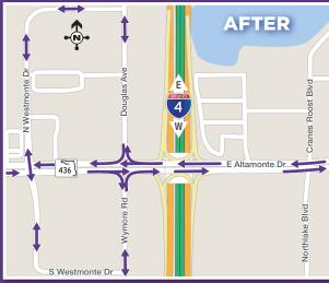
Removing the traffic signal at S.R. 436 and Wymore Road/Douglas Avenue and redirecting traffic to Westmonte Drive provides more capacity for vehicles exiting I-4 and improves traffic flow. Wymore Road and Douglas Avenue will become a right-in, right-out only from S.R. 436. Improvements, including additional turn lanes at S.R. 436, will be constructed on Westmonte Drive.
