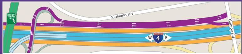
I-4 Ultimate improvements at the Florida's Turnpike interchange will foster better traffic flow and create a safer merging environment. The separate three-lane auxiliary ramp and limited entry points eliminates free merging between westbound I-4 and Conroy Road on-ramp. Those entering westbound I-4 from Conroy Road will continue through the auxiliary lanes and eventually merge into I-4. The additional lanes on the Florida's Turnpike ramps allow for greater motorist capacity.
