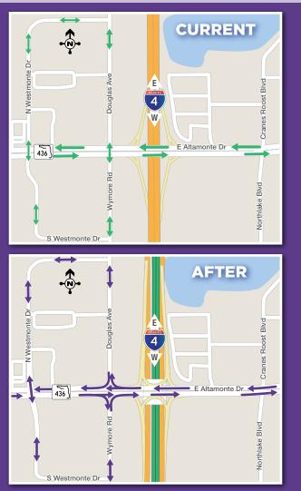
Removing the traffic signal at S.R. 436 and Wymore Road/Douglas Avenue and redirecting traffic to Westmonte Drive provides more capacity for vehicles exiting I-4 and improves traffic flow. Wymore Road and Douglas Avenue will become a right-in, right-out only from S.R. 436. Improvements, including additional turn lanes at S.R. 436, will be constructed on Westmonte Drive.
