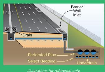
Illustrations for reference only. Final design is subject to change. vibratory pile driving, excavate the site, and finally install the system — all while continuously operating a de-watering pump.
